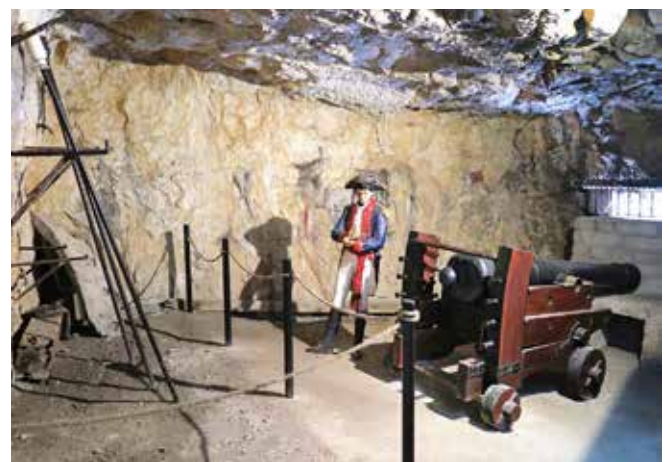
Cornwallis Chamber: one of two gun positions – both modified in WWII – with a reproduction Koehler Depressing Carriage (1782) which enabled the British to fire on the Spanish lines at depression angles of between 20–70 degrees. Photo Clive Penfold
